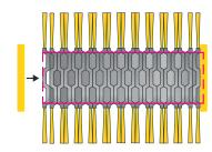
3. The final brush ring assembly should resemble the example shown below.
